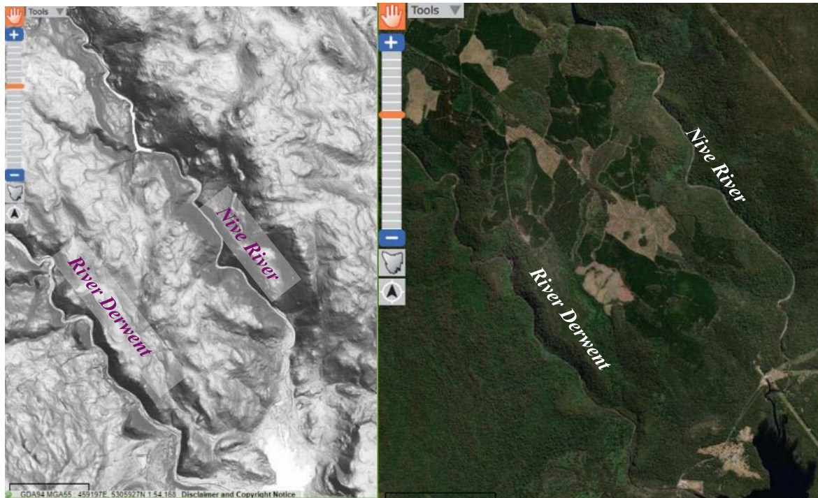
Figure 6.50: (left) Lidar image of the Nive River between Lake Liapootah and Wayatinah Lagoon showing the incised valley widening upstream of the downstream lagoon. The incised River Derwent is also shown. Aerial image of the Nive and River Derwent showing forestry activities and Wayatinah Village (right).
