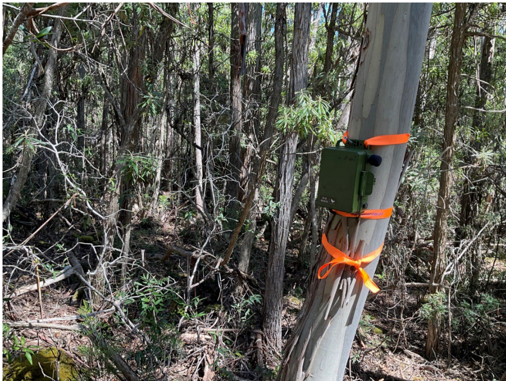
Figure 6.3: Wildlife Acoustics Song Meter SM4 acoustic recorder deployed in Tarraleah Conservation Area
