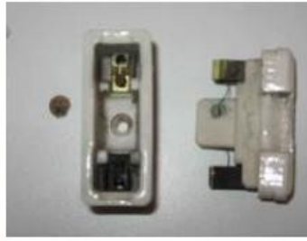
Poor rewirable fuse wedge contact
