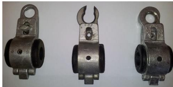
Older style clamp Older style clamp with failure Current clamp with reinforcement
