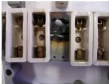
Failed active bus on federal switchboard
