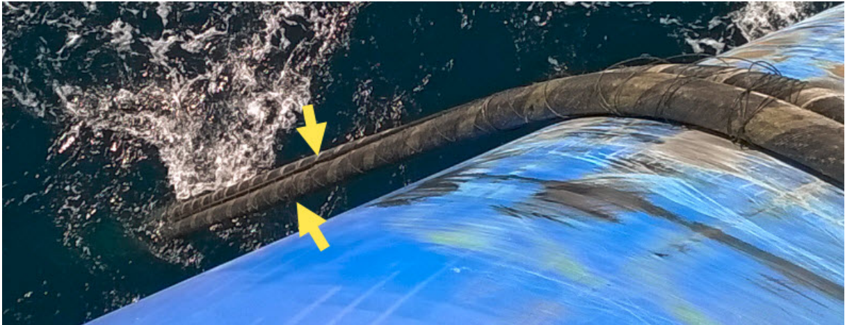
Photo 1. Fault coming aboard indicated by bulges in the outer serving (arrowed)
