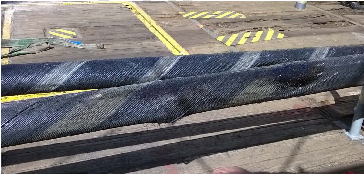
Photo 2. Main bulge at fault and secondary bulge nearby oozing compound.
