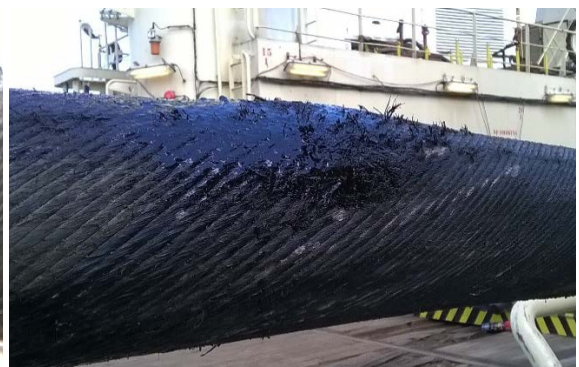
Photo 6. Secondary bulge oozing compound
