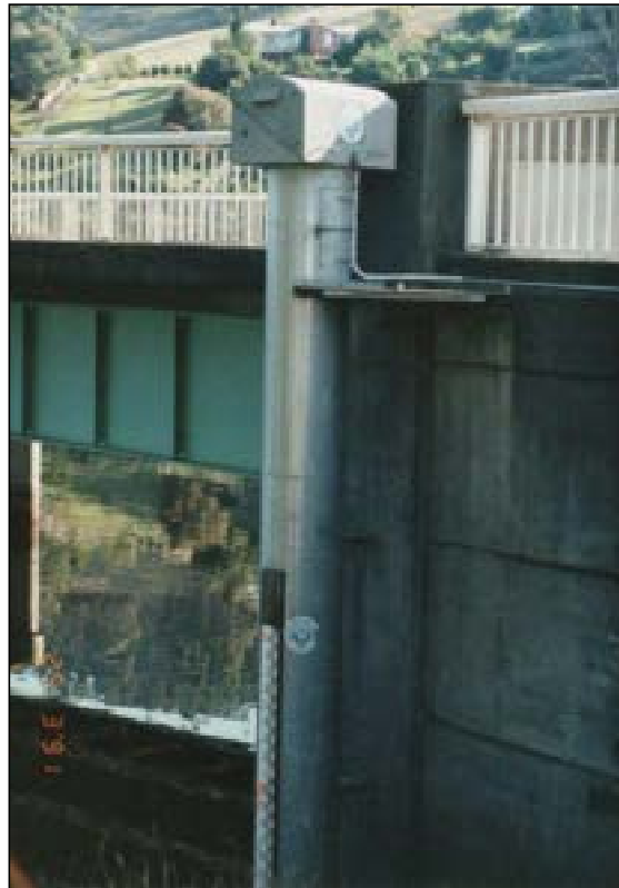
Figure F.3: Huonville flood gauge located on the left bank (looking downstream) on the downstream abutment (0m at the gauge = -1.438m AHD)
