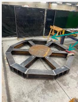
Slings attached to frame for original tilt, sling guards not used.
