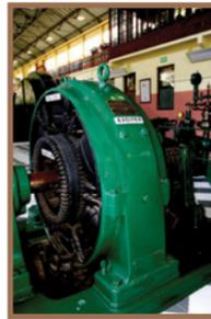
The exciter at Waddamana A was started by a mini turbine. It was also used for emergency power supply at the power station when normal power supplies were cut off.
