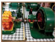
At Waddamana A two machines were initially installed. Each had a capacity of 4 900 horse power (HP) (3.65 MW) enough electricity to supply about 250 to 300 homes. They came into operation in 1916, at that time there were about 2000 customers in the Hobart area. An additional machine was operating by 1919. A further six 8 000 HP (5.96MW) machines were installed after 1922.
