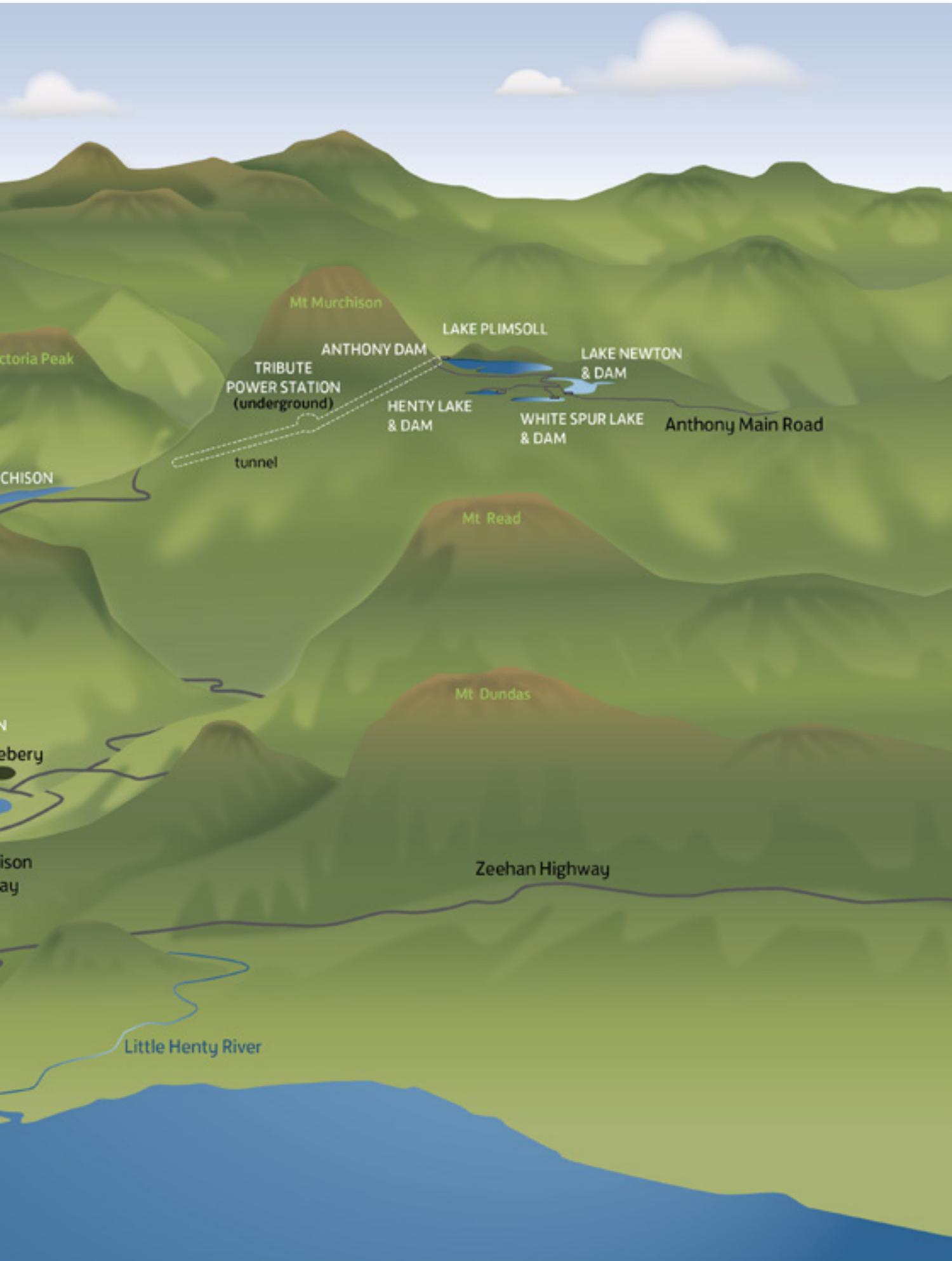
Figure 4: Schematic representation of the Anthony–Pieman hydropower scheme
