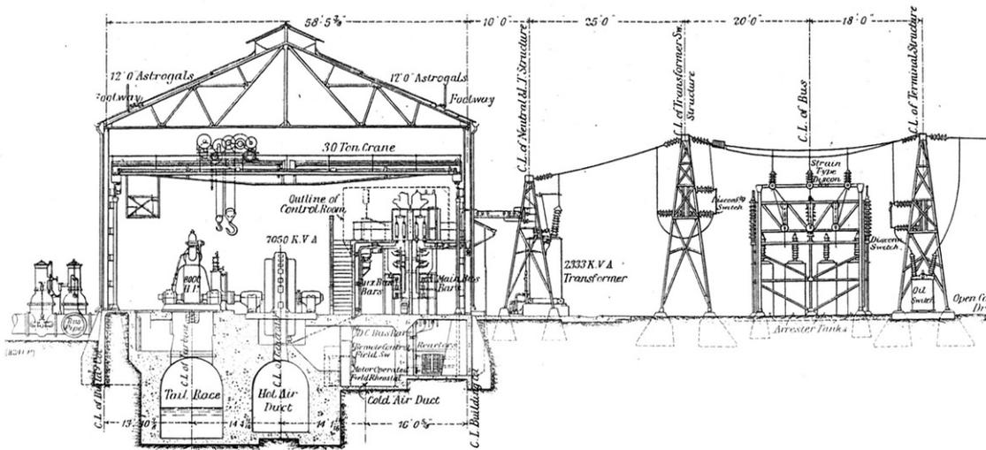
Figure 2.6 Section of Waddamana A (c1924) (Engineering based on an official plan).
