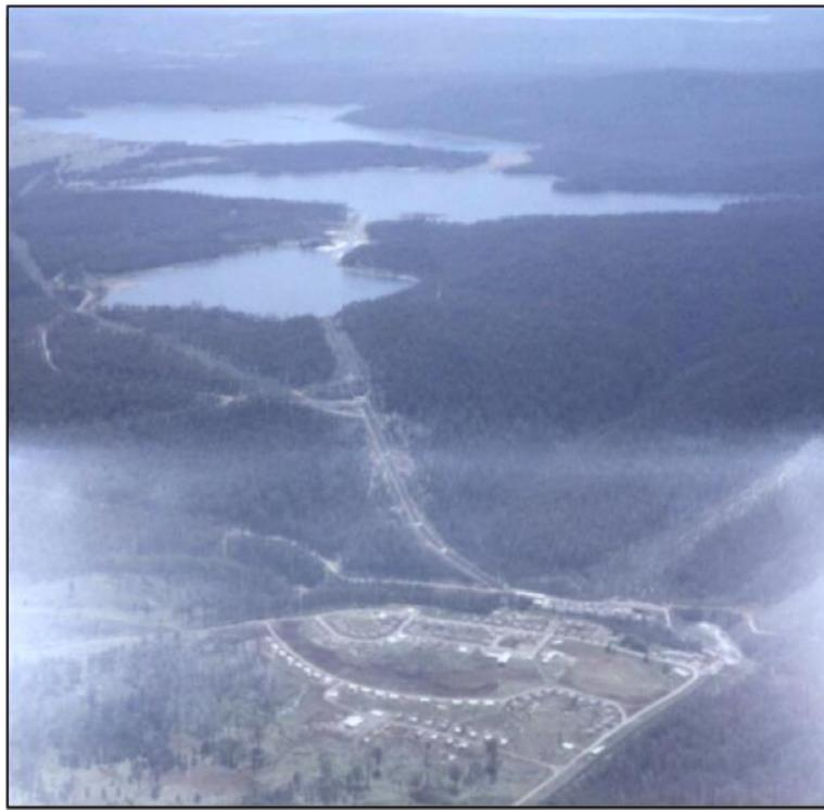
**Figure 2.5: Overview of the Tungatinah power development in 1957, showing interconnected canals, pipelines, man-made lakes, dams and associated Bronte village.<sup>42</sup>**
