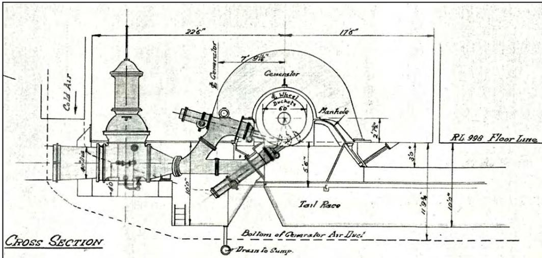
Figure 19: Cross section of Boving & Co. turbine in plans for Tarraleah Power Station (HEC - DW145 vol 1 Tarraleah Power Station 1935-37).
