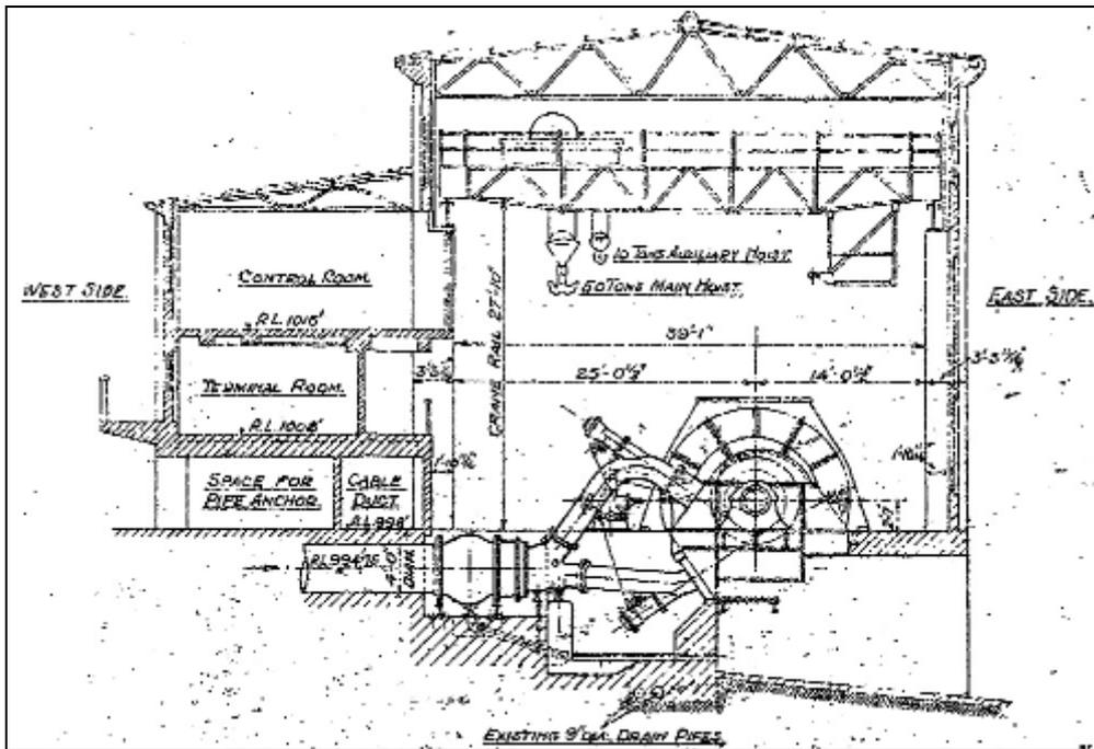
Figure 29: Section of building showing English Electric Co machine, crane and rooms to the west (HEC plan – O/6026).
