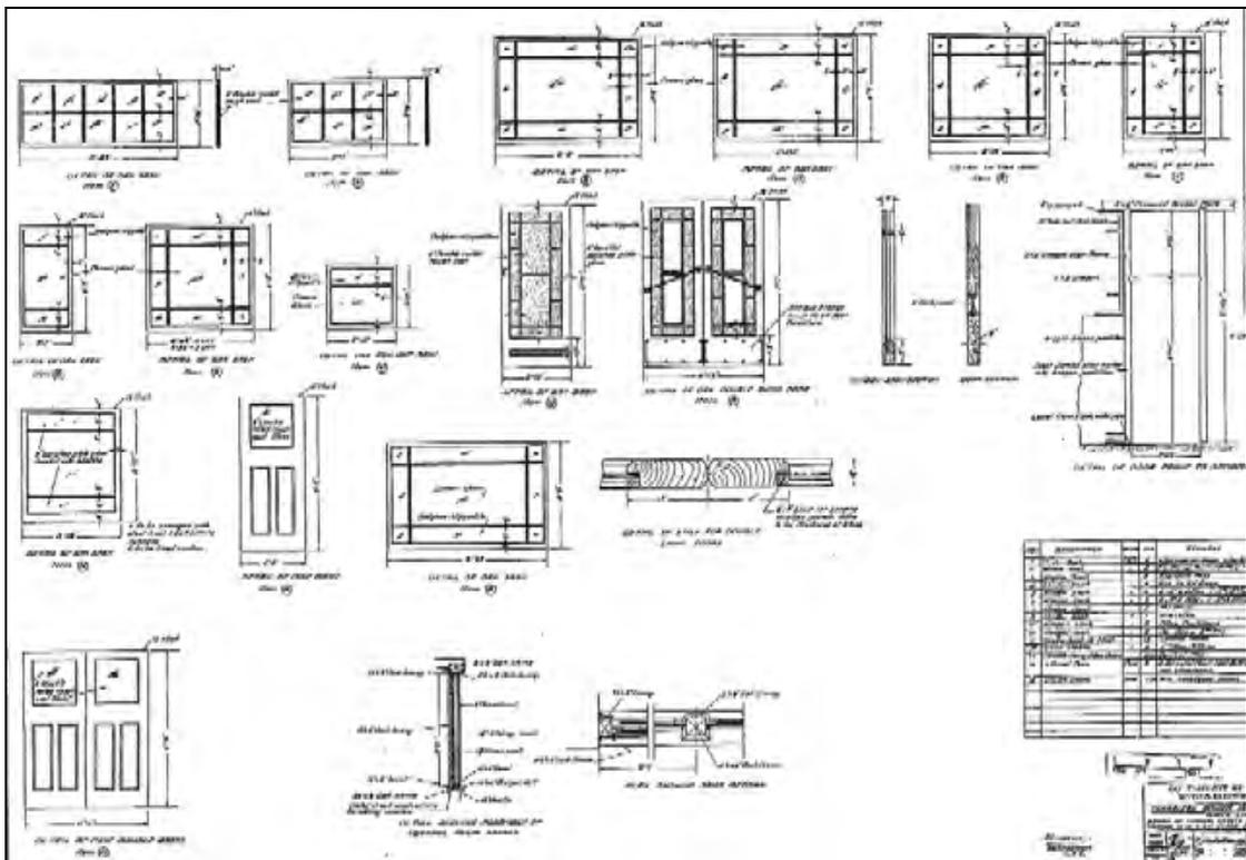
Figure 10: Details of doors and windows in second floor offices of power station (HEC plans - A5489).
