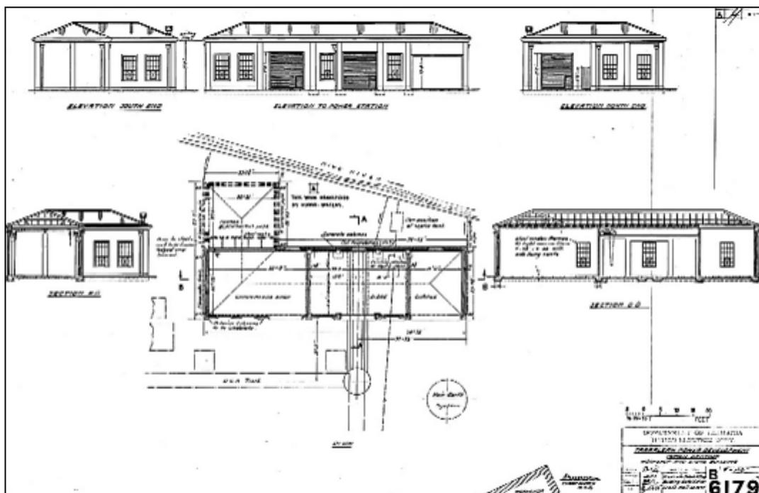
Figure 12: Plan and elevations of workshops and garage/store adjacent to the switchyard showing blacksmith's wing, which was washed away in the 1939 floods (HEC plans - B6179).
