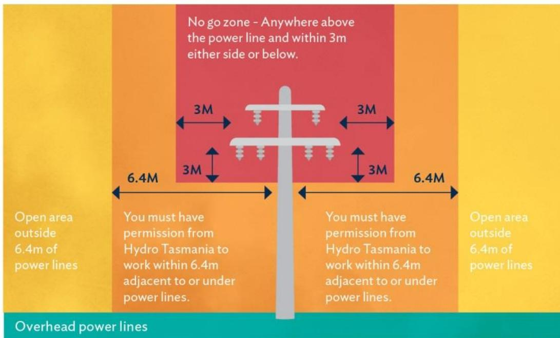
**Figure 3: Working near overhead power lines**
