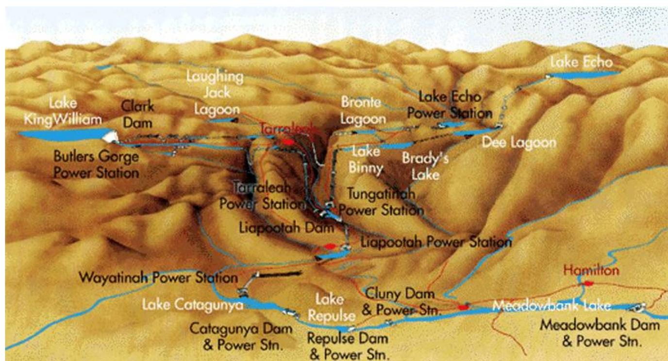
**Figure 2:** Derwent cascade system of dams and power stations
