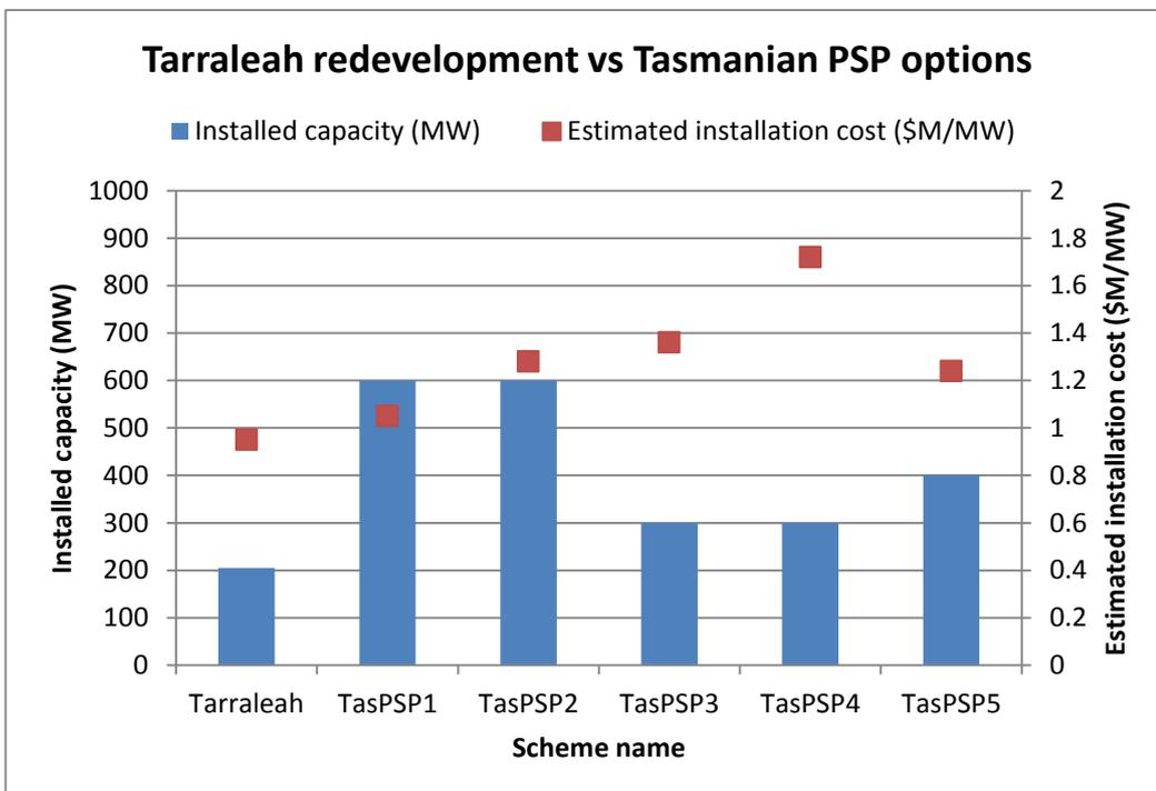
Figure 4: Tarraleah redevelopment vs Tasmanian PSP options – installed capacity and estimated installation cost
