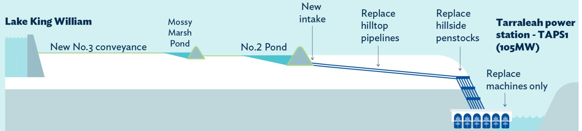
Figure 15: Maintain existing station option diagram
