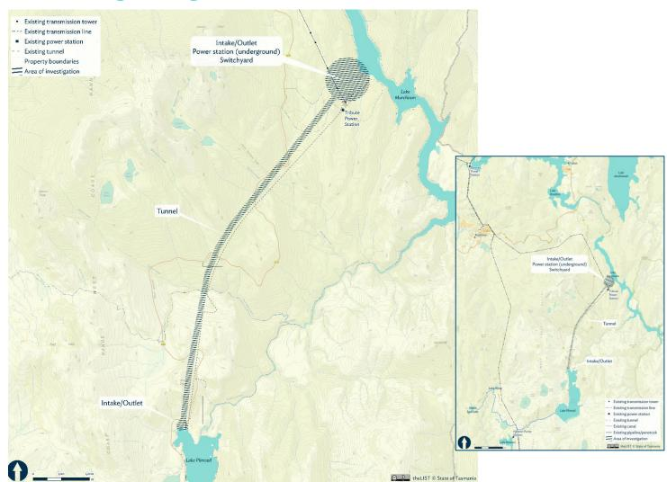
The potential pumped hydro development near Tribute uses two existing storages – Lake Plimsoll as the upper storage and Lake Murchison as the lower storage. This option involves:
