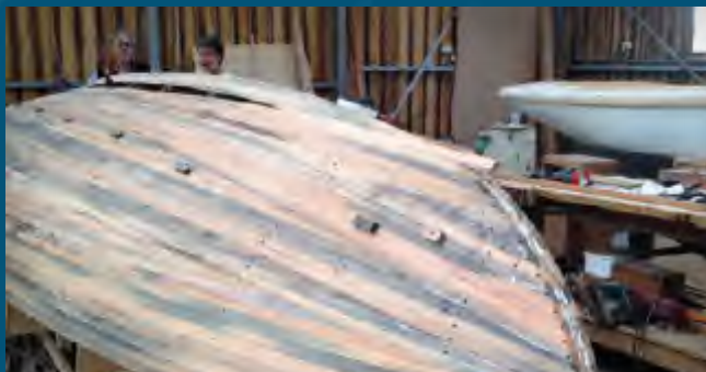
Boat builders Andy Gamlin and Peter Heading work on Pipe Dream , built with salvaged King Billy Pine. Photo courtesy ABC TV
