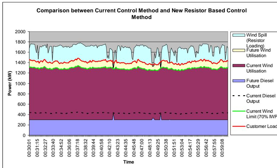
Figure 1: Comparison between current control method and new resistor control method
