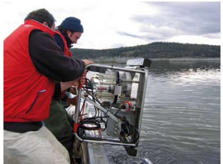
Geoff Nicholson (Marine and Freshwater Research Institute, Victoria) and John Sherwood (Deakin University) deploying a benthic chamber to measure nutrient release from the sediment at Lagoon of Islands
